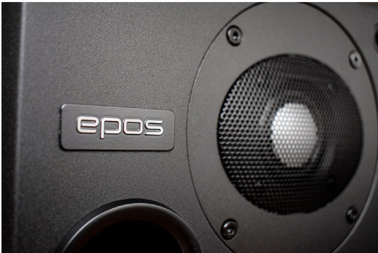
The tweeter of the Epos 7N with its 28 mm ceramic-coated dome tweeter already shone in the „big“ Epos 14N (Photo: H. Biermann)
