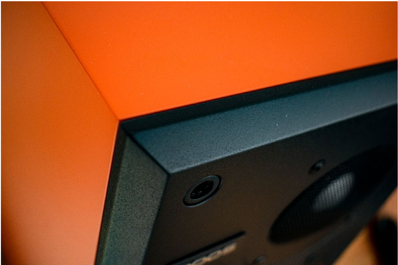
The picture shows the good paint quality and the attached baffle, which is slightly chamfered at the edges for acoustic reasons (Photo: H. Biermann)
